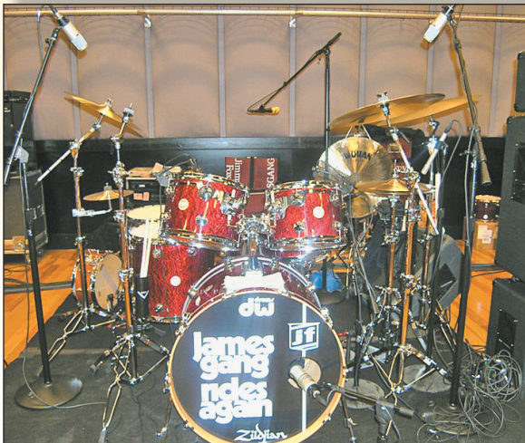
The 100 watt guitar amp is less than 2' from the right PR 30 over the cymbal but with the incredible rear rejection of the Heil PR 30 that guitar was hardly detected in the overhead channel!
