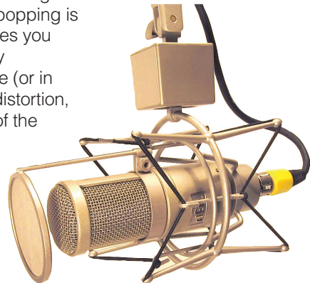
Heil PR 40 in the SM2 shock mount shown with the BSW “pop” filter.
